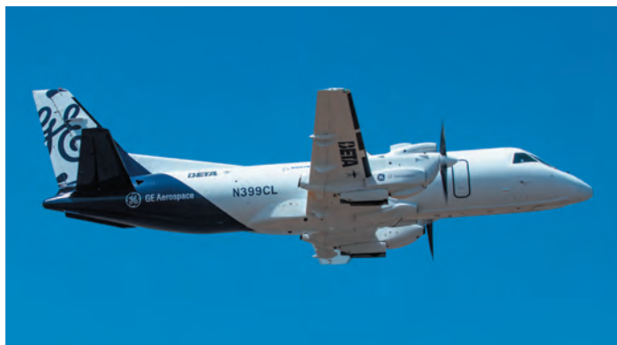
GE Aerospace SAAB 340B Hybrid Testbed – GE Aerospace SAAB 340B hybrid-electric demonstrator demonstrating megawatt-class hybrid-electric propulsion in flight.
