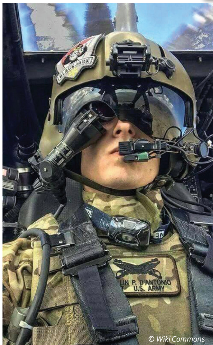
The AH-64 Apache's Integrated Helmet and Display Sighting System (IHADSS) represented a major step in cockpit evolution, projecting flight and targeting information directly into the pilot's field of view while linking head movement to the helicopter's sensor and weapon systems.
